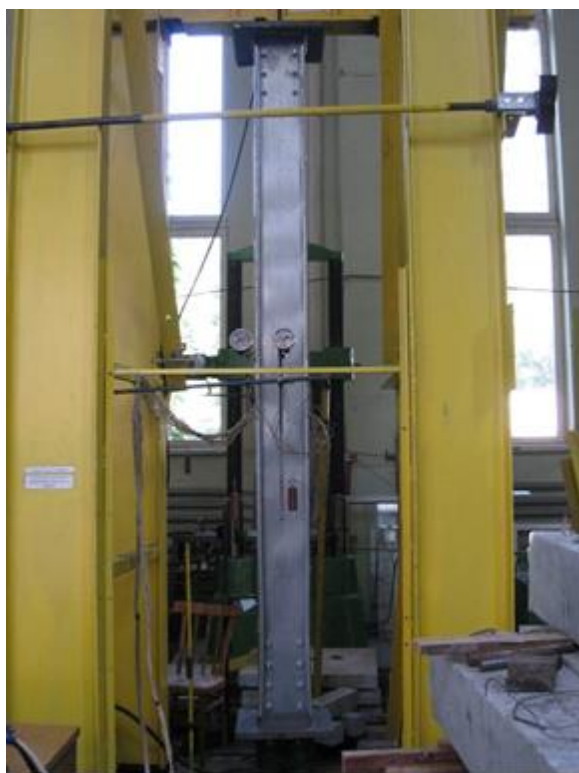
Fig. 1. Experimental test of the column made of thin-walled bending profiles.
