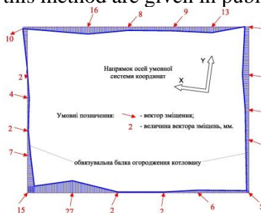
Fig.5 – Curve of horizontal movements that occurred during lifting
